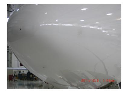
Photograph of the nose radome of the GV, showing three of the five pressure ports used to determine flow angles as part of the gust-measuring system:
