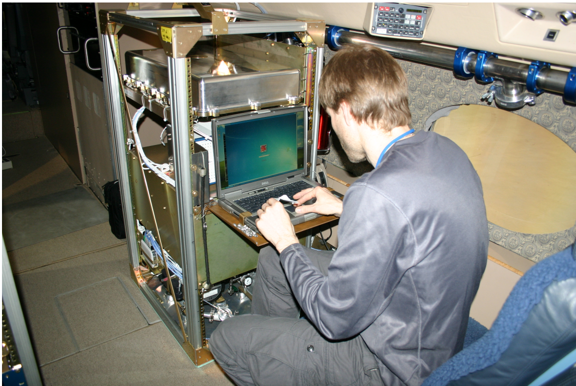
Figure 1: Petter Weibring operating the CAMS instrument on the GV. The optical system, including the lasers, detectors, multipass cell and other components are mounted in the Aluminum covered enclosure near the top.
